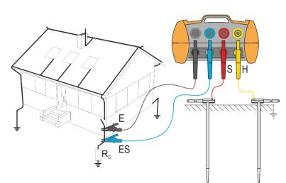
Test leads should be connected to the measurement terminals in the device, as shown above.
