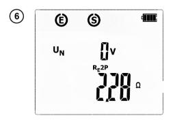
After the measurement, its result is shown: at the bottom of the screen, the main result is shown for  $R_E 2P$ , whereas the upper part of the screen shows the measured interference voltage  $U_N$ . The result is displayed for 20 seconds. The result can be recalled by pressing ENTER button.
