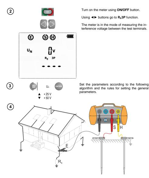
Test leads should be connected to the measurement terminals in the device, as shown above.
