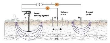
The scheme of measuring the earthing resistance with the 'technical method' is shown above. The figure shows the measurement of earthing resistance  $\mathbf{R}_{E}$ . To perform the measurement, use two additional auxiliary electrodes:
