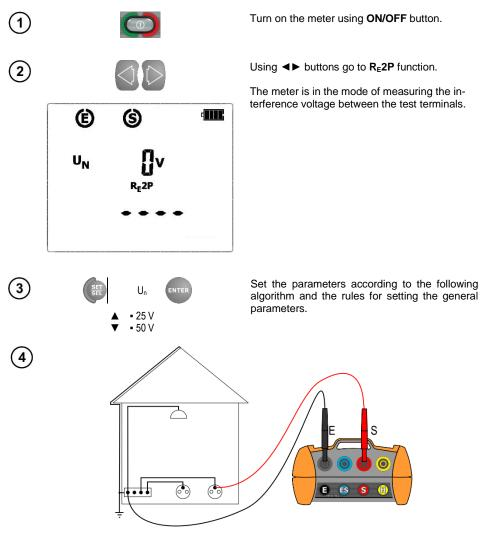
Test leads should be connected to the measurement terminals in the device, as shown above.
