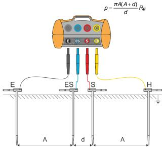
Connect the four aligned auxiliary electrodes, which are driven into the ground, to the meter, and do so in accordance with the diagram. The distance between electrodes E and ES, as well as between S and SH are equal to each other, and at the same time is greater than or equal to 3 times the distance between electrodes ES and S (A  $\ge$  3·d).
