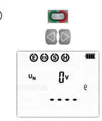
Turn on the meter using **ON/OFF** button.
