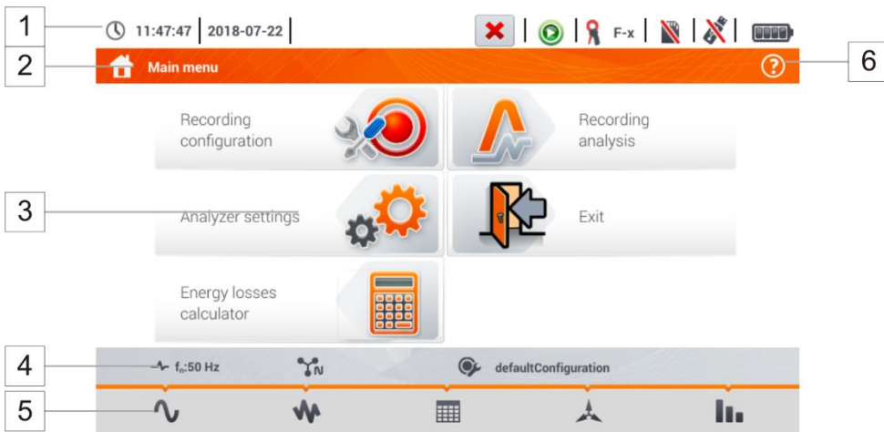
Fig. 5.2 Main elements of the recorder screen
