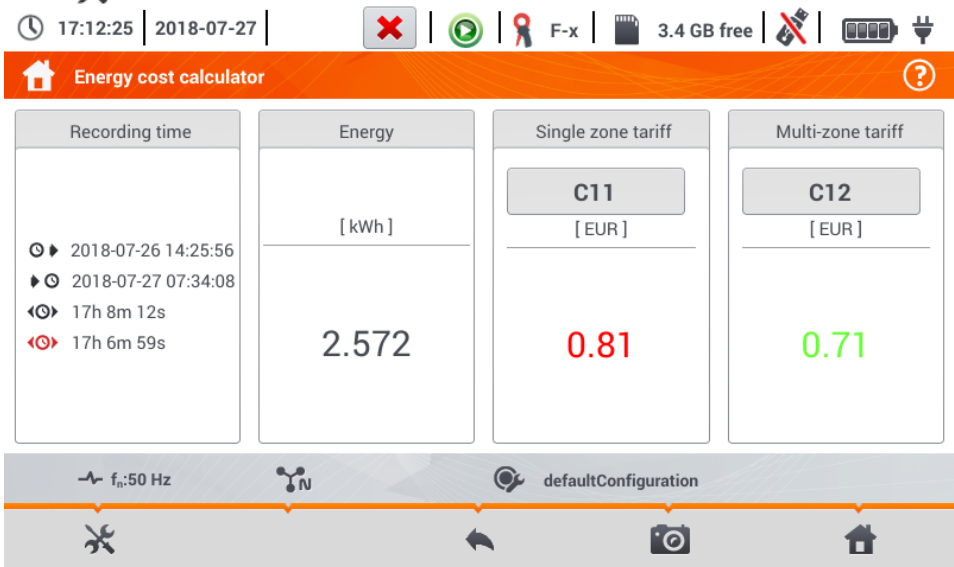
Fig. 5.28. Screen with indications of the energy cost calculator
