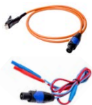
Test lead 1.8 m (crocodile clip) WAPRZ1X8ORKS PAT-96 | 1.5 m (PAT plug/banana plugs) WAPRZ1X5DZBB
