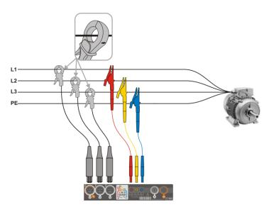
Fig. 5.6 Wiring diagram – 3-phase with three operating wires
