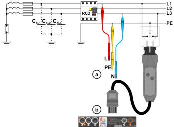
Fig. 3.7 RCD measurement in the IT network. The circuit is closed by the parasitic capacitances C<sub>x</sub>
