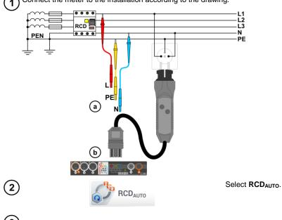
Connect the meter to the installation according to the drawing.
