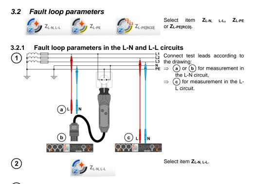
(3) Select other settings and perform the measurement using the START button on the device.
