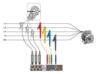
Fig. 5.5 Wiring diagram – 3-phase with four operating wires
