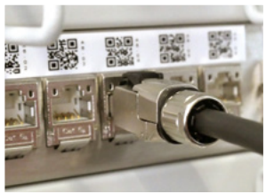
Before testing, scan the label with WireXpert MP
