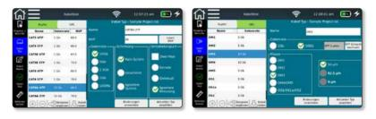
**Important:** Before running a test, it is necessary to select the correct type of cable, otherwise the result could be affected.
