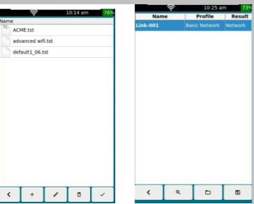
"Site&Data" shows the currently selected directory for saving data and the names of the current and next test. Click on "Site" shows the list of tests in the current directory and allows to create a new "Site" and switch between "Sites".
