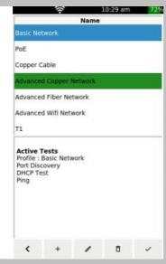
"Profiles" shows the currently selected test profile and the main settings of the profile. Click on "Profiles" opens the "Profiles" menu to change or create new profiles.
