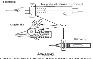
Barrier is a part providing protection against electrical shock and ensuring the minimum required air and creepage distances. Always keep your fingers behind the barrier during a measurement.
