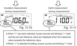
and the pre-set reference value are displayed when the measured value is less than the reference value.
