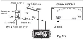
(6) Press the TEST button or remote control switch to start a continuous measurement.
