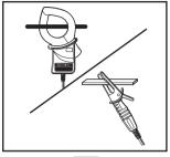
Clamp on the measured object and fix the Sensor. Firmly fix it so as not to easily come off.
