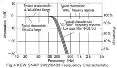
Note: Characteristic of -24dB/octiave means that signal magnitude declines to about one sixteenth of that at the initial frequency when frequency doubles. KEW SNAP 2432 and KEW SNAP 2433 have the following two settings for the Frequency Selector Button.
