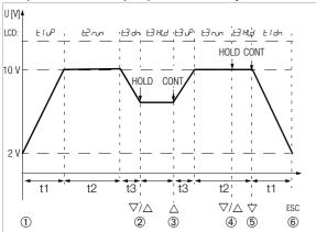
**Ramp parameters:** output quantity: U (range of 0 ... 15 V),  $5 \pm Rr \pm 2$  V, Erd = 10 V, Erl = 5 S, Erl = 8 S, Erl = 5 S. Ferl = 8 S, Erl = 8 S, Erl = 8 S. Er
