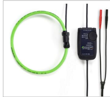
Flexible current clamp sensor for selective earthing resistance measurement
