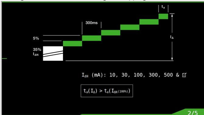
And thus both tripping current and tripping time are measured and displayed.
