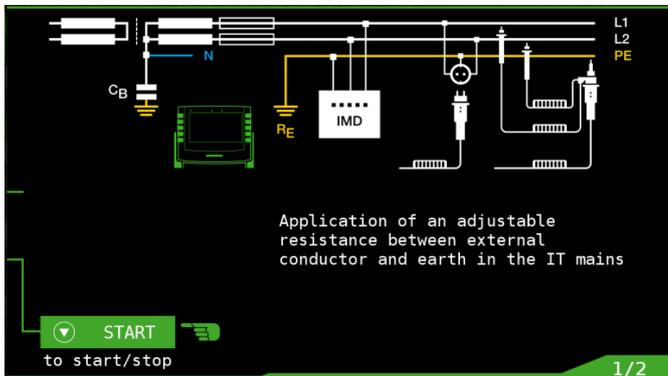
Insulation monitors can be tested with the help of this special function. After pressing the START button, an adjustable insulation resistance is activated between one of the two phases of the IT system to be monitored and ground to this end. This resistance can be changed in the manual sequence mode with the help of the softkeys, and it can be varied automatically from  $R_{max}$  to  $R_{min}$  in the automatic operating mode.
