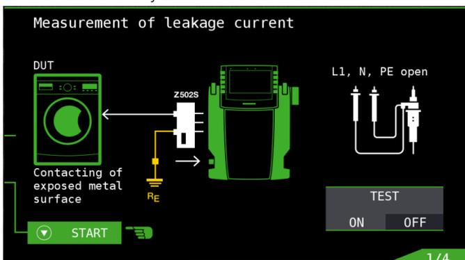
As specified in the standards listed above, current values of up to 10 mA can be measured with this measuring adapter.
