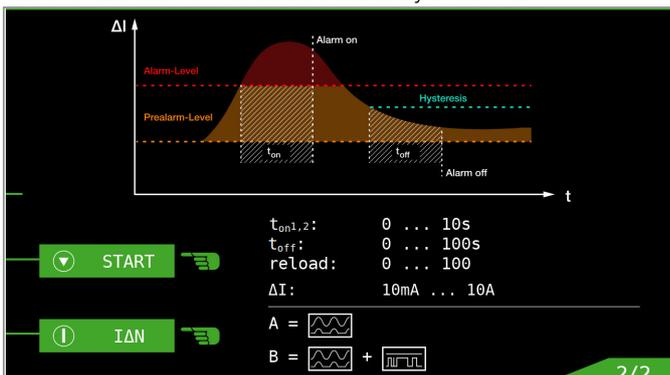
If an RCM is used in combination with an external switching device, the combination must be tested as if it were an RCD.
