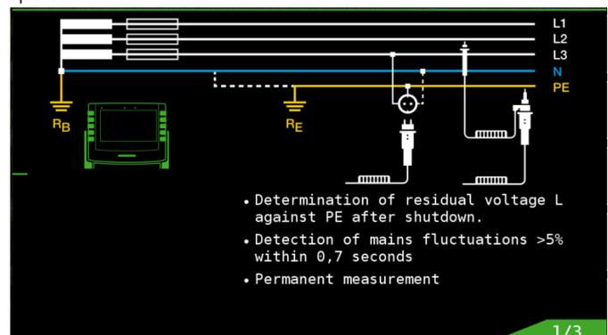
With the PROFITEST MF XTRA, testing for the absence of voltage is performed as follows by means of a voltage measurement which involves measuring discharge time  $t_U$ :
