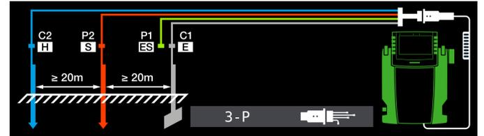
4-wire measuring method, probes and earth electrodes connected via PRO-RE adapter
