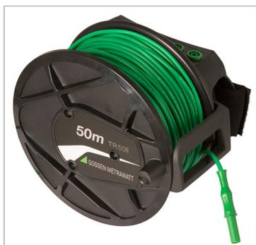
50 m measurement cable coiled onto a plastic reel. Connection to the inside end of the cable is made possible with two sockets integrated into the reel. The other end is equipped with a banana plug. Cable resistance can be compensated for with the rotary selector switch in the  $R_{LO}$  position.
