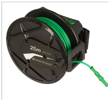
25 m measurement cable coiled onto a plastic reel. Connection to the inside end of the cable is made possible with two sockets integrated into the reel. The other end is equipped with a banana plug. Cable resistance can be compensated for with the rotary selector switch in the  $R_{LO}$  position.
