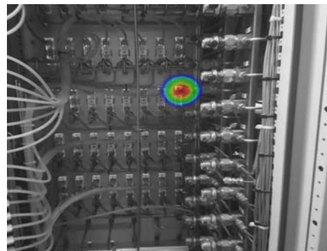
Like thermal imaging (left), acoustic imaging (right) uses the wavelengths emitted by an object to locate and measure defects. Thermal imaging uses invisible light wavelengths, while acoustic imaging uses inaudible sound wavelengths.
