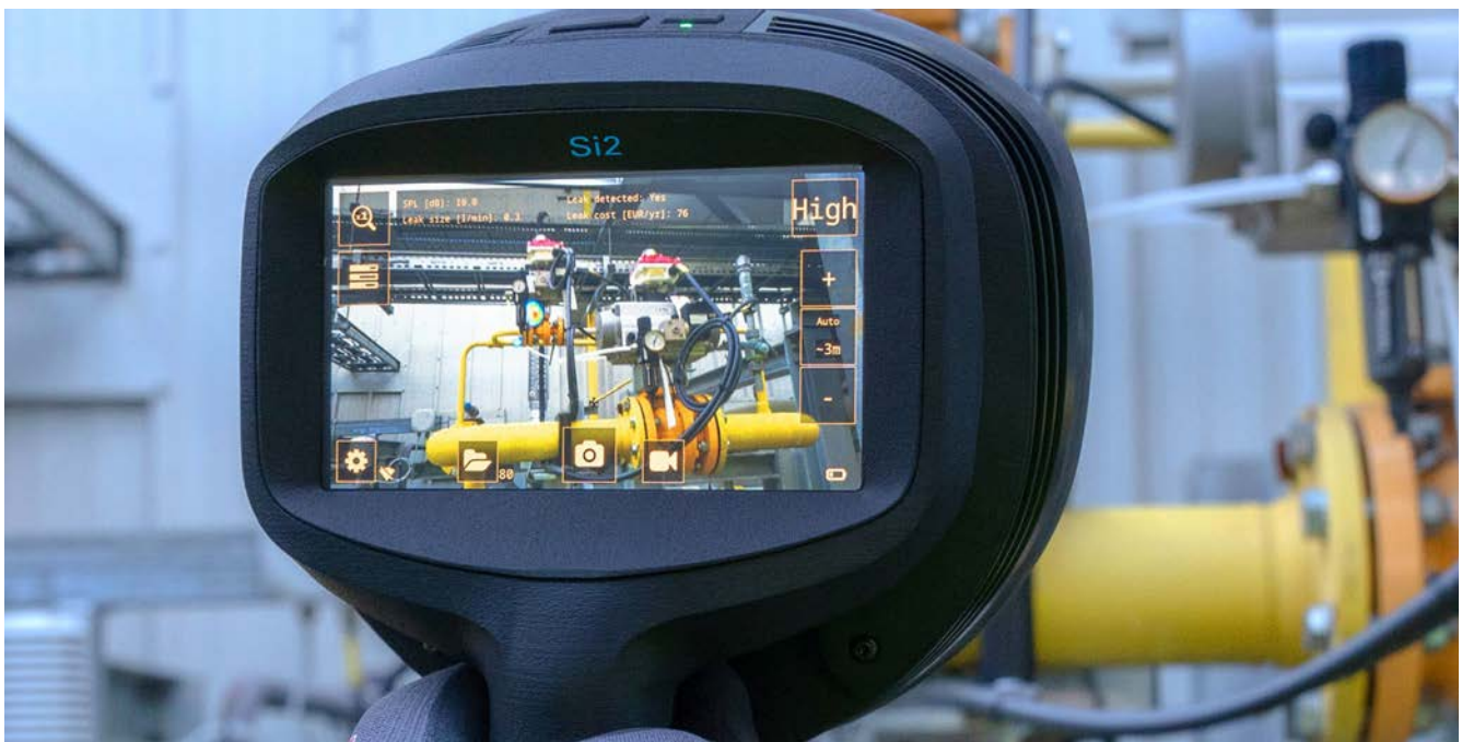
FLIR Si2 leak detection acoustic imager in the field calculating leak size and cost of leak.
