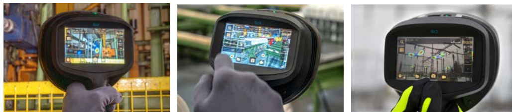
Ultrasound cameras showing, from left to right: compressed air leak, mechanical fault, and partial discharge.
