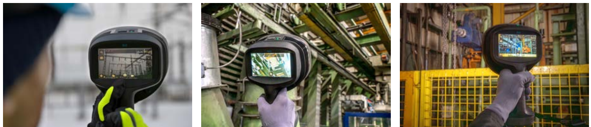
The FLIR Si2 camera detects, assesses, and measures electrical faults, mechanical issues, and air and gas leaks.
