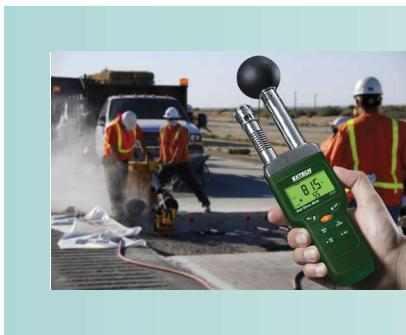
**Extech's Heat Stress WBGT (Wet Bulb Globe Temperature) Meter** accurately determines the Heat Stress level (how hot it feels outside) by factoring a combination of humidity, temperature, air movement, and direct solar radiation. These factors all affect how hot our bodies get, as well as our ability to cool down. It's perfect for monitoring the Heat Index on hot humid days to prevent heat stroke during road or building construction, outdoor activities, sporting events, or in the workplace.
