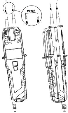
**Test Probe Storage on Back Side**
