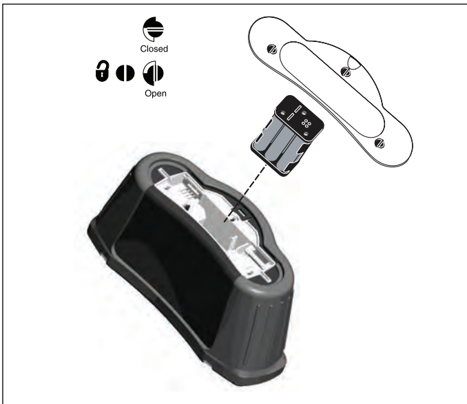
Figure 24. Replacing the Batteries
